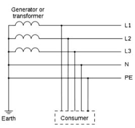
connected to earth via this earth point on the source side. See fig. below which depicts this:
