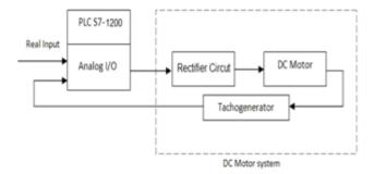
Figure 1: System block diagram.
